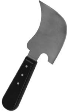
T117 Crescent Shaped Knife: Used for trimming welding rod flush with the flooring surface. It is also used in conjunction with the Trim Plate.
