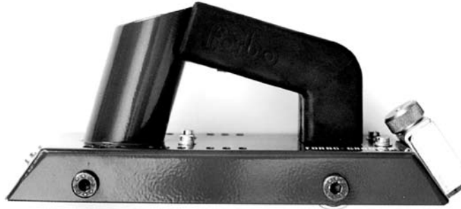
T133 Forbo Groover: A push groover used for correctly grooving out seams in linoleum and homogeneous vinyl for heat welding. It uses the T206 blade, which is the same blade used for the hand groovers for a consistent groove throughout.
